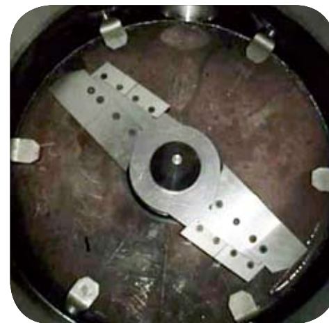
Inside the cell: fixed and rotating blades
